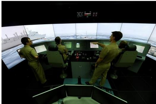
**The Littoral Combat Ship Full Mission Bridge** is a full sized trainer that students with orders to LCS ships can train on in preparation of reporting to their new command. Using the same software as FMB and COVE, the LCS trainer has every Navy homeport modeled and allows LCS student to navigate in and out of designated ports using the highly sophisticated controls of a real LCS. The LCS Bridge trainers are installed at SWOS Newport and at the Mayport and San Diego LTFs
