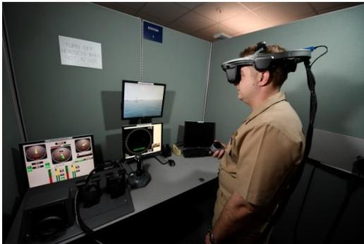
**COVE I** stations are used primarily for BDOC and ADOC students. These stations consist of a virtual reality (VR) helmet that gives them a 360-degree view of their surroundings. Using a state of the art voice recognition system, students can give commands to the virtual helmsman, which are repeated back by the computer. SWOS employs 36 x COVE I stations across the domain: 9 at BDOC Norfolk, 9 at BDOC San Diego, and 18 at SWOS Newport. NSTC
